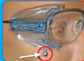
Left: A B-26+ ® SideShield successfully deflecting a 1/4 inch steel ball at 150 fps (102 mph) during testing.
