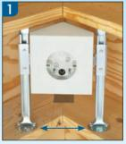
For proper fan/fixture installation, use supplied template to level and position brackets between rafters. Remove captive screws on sides of brackets and use to attach FBX900 assembly to rafters.
