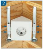
Loosen the screws noted above. Slide box to center it between rafters. Tighten screws. Install wires.
