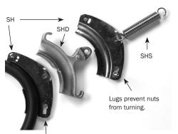
Keyhole slots permit assembly on cable without removal of bolts or threading of cable through fitting.
