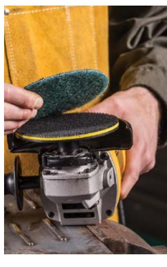
Max RPM is determined by corresponding back-up pad.
