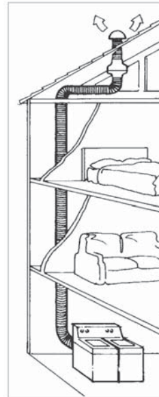
(In-Line) Fan assisted dryer exhaust
