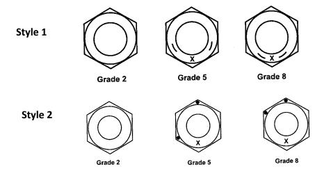
**Notes:** Marking can be Style 1 or Style 2. The nuts will also have manufacturer's marking on the head in addition to the grade marking as shown above. Grade 2 nuts will not have any markings (both grade and manufacturer's marking).
